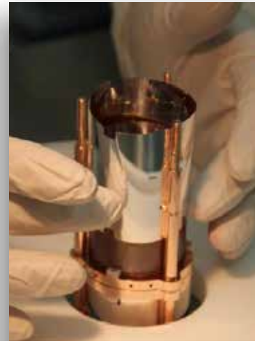
#2 ZnSe and light reflector installation
